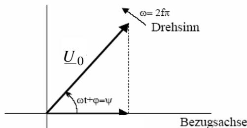
$$\underline{U}_0 = \text{Re}(\underline{U}_0) + j \text{Im}(\underline{U}_0) = U_0 (\cos(\varphi_0) + j \sin(\varphi_0)) = U_0 e^{j\varphi_0}$$
