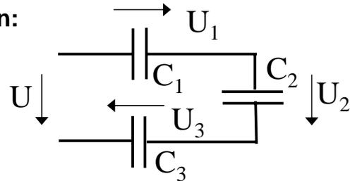
$$U = U_1 + U_2 + U_3 = \frac{1}{C_1} \int_0^t I dt + \frac{1}{C_2} \int_0^t I dt + \frac{1}{C_3} \int_0^t I dt = \left( \frac{1}{C_1} + \frac{1}{C_2} + \frac{1}{C_3} \right) \int_0^t I dt$$
