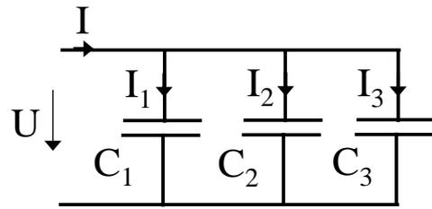
$$I = I_1 + I_2 + I_3 = C_1 \frac{dU}{dt} + C_2 \frac{dU}{dt} + C_3 \frac{dU}{dt} = (C_1 + C_2 + C_3) \frac{dU}{dt}$$
