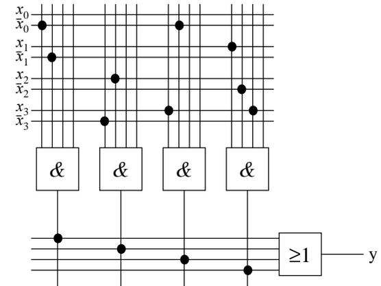
$$f(x_3, x_2, x_1, x_0) = \bar{x}_1 \bar{x}_0 \vee \bar{x}_3 x_2 \vee x_3 \bar{x}_0 \vee x_3 \bar{x}_2 x_1$$
