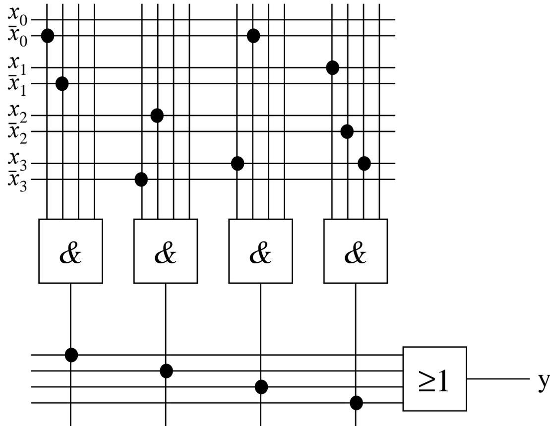
$$f(x_3, x_2, x_1, x_0) = \bar{x}_1 \bar{x}_0 \vee \bar{x}_3 x_2 \vee x_3 \bar{x}_0 \vee x_3 \bar{x}_2 x_1$$
